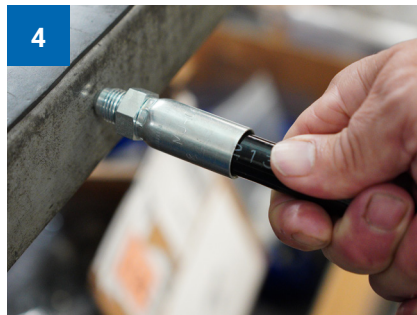
Push coupling to the marked insertion depth.
