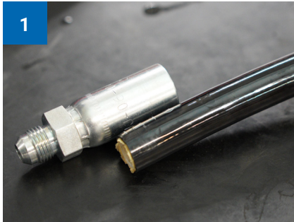
Establish hose insertion depth using the coupling you're going to swage.
