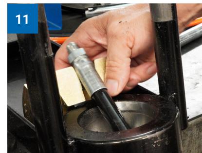
Release the pressure valve, remove die and hose from base. (Spray wax or engine assembly lube will help coupling release)
