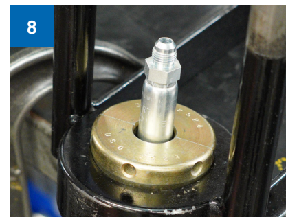
Next, insert the second die half into the die base.
