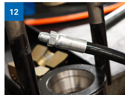
Inspect assembly for gaps between the hose and coupling. Repeat steps 5 - 10 using a smaller die set if needed.
