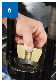
Install the first die half in the machine base.
