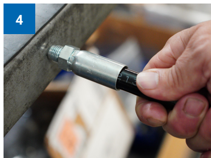
Push coupling to the marked insertion depth.
