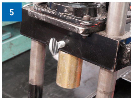
Install the pusher into the pusher block and tighten the thumb screw
