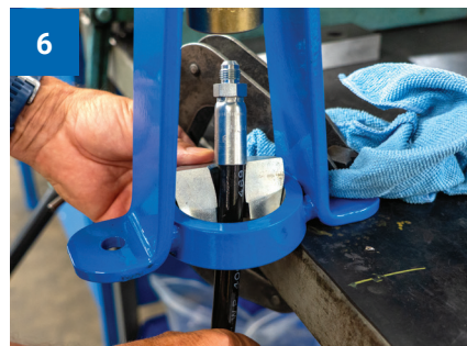
Install the hose assembly up through the base and into the pusher.
