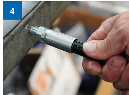
Push coupling to the marked insertion depth.
