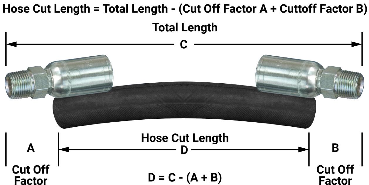
2. Squarely cut the hose length required, clean the I.D. of the hose, and remove loose wires etc. from cut ends. Then using the reusable shell, mark the insertion depth required on the O.D. of the hose using the paint marker or marking tool.
